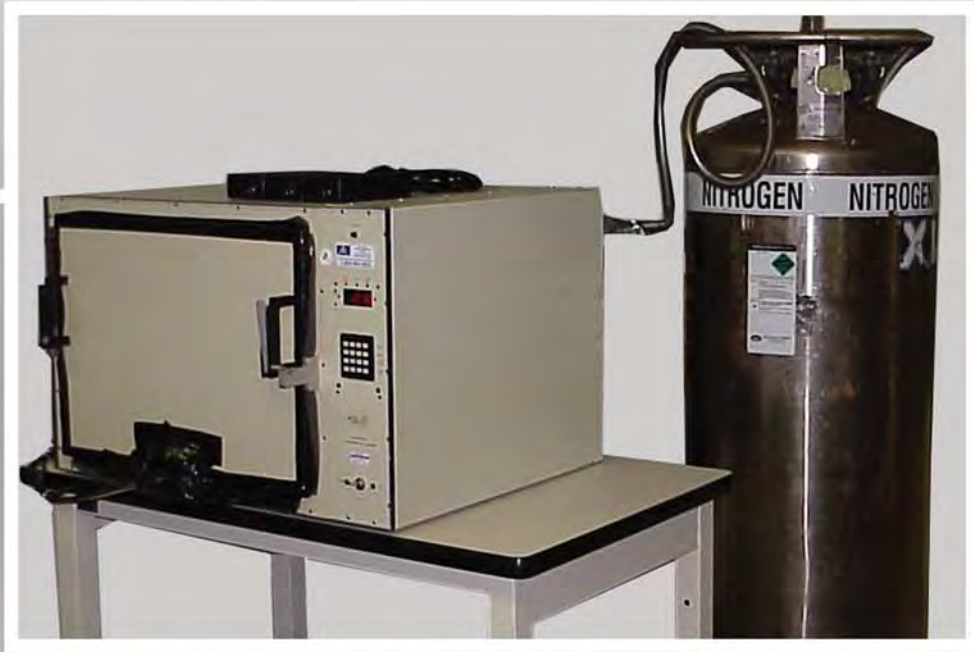
Close-Up of Thermal Chamber and Liquid Nitrogen tank
