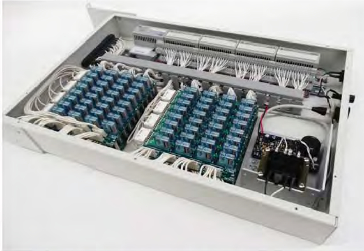
Power Matrix Unit (Dual 32x4 15A Matrices)
