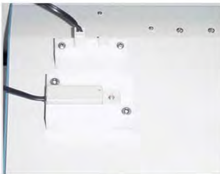
Encapsulated Thermocouple installed in Test Fixture
