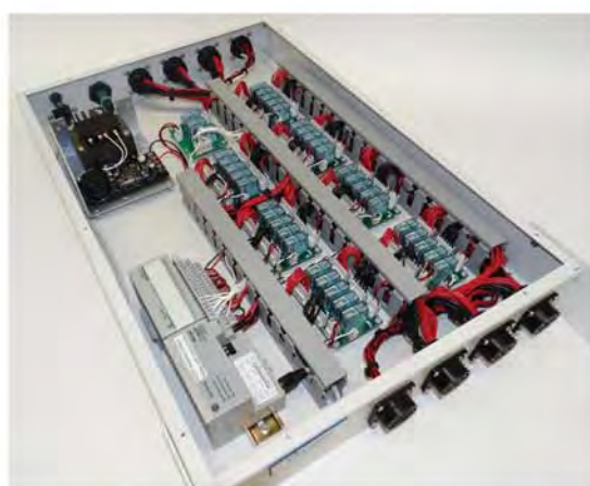
Programmable AC/DC Control Unit
