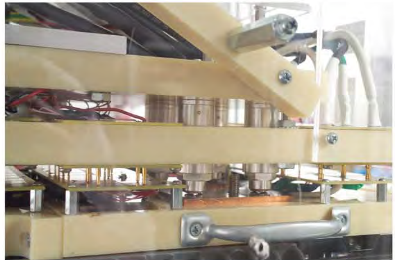
Close-Up of High Current Pogo-Pins
