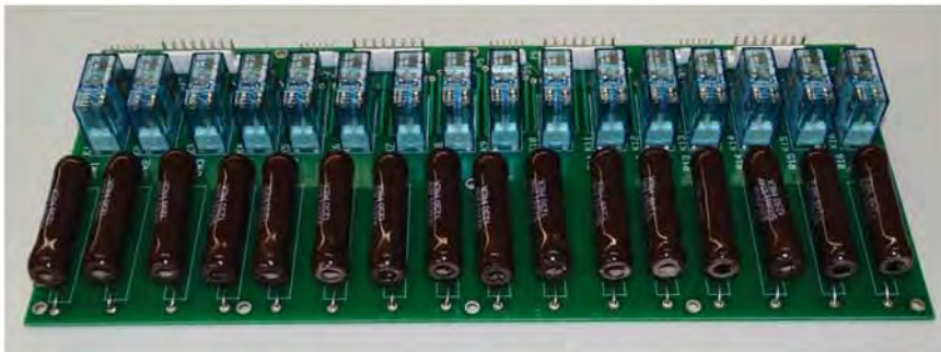
Close-Up 5k Min Load Resistor Load Board
