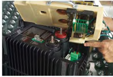
using Pogo-Pins, LED sensors & Bus Bars
