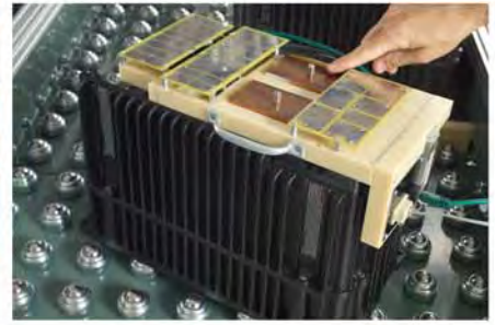
Bus Bars and large PCB Pads for Test Fixture Pogo-Pins
