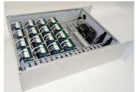
5k Min Load Unit with multiple Resistor Boards
