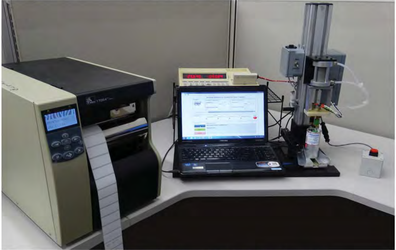
Front view of System with Label Printer, Computer, LCR Meter and vertical Air Cylinder to connect to UUT
